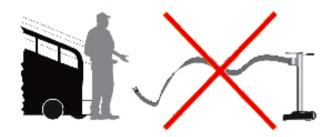
**6. DO NOT** release the belt end with unassisted retraction. **DO NOT** drop the belt end.
