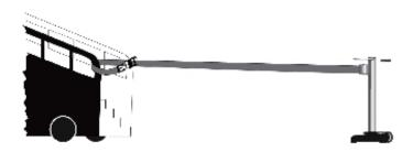
**3.** Loop the belt end through a stationary object and secure the belt end back onto itself to create a temporary barricade.
