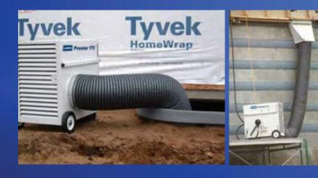
Certified to ANSI Z83.7 and CSA 2.14 standards for safety and rated for indoor-outdoor use. Flexible setup and an even, steady heat delivery make Premier heaters well-suited to many applications from framing, drywalling, stucco work, construction enclosures, brick and block laying, freeze protection, bridgework, docks to excavation and more.
