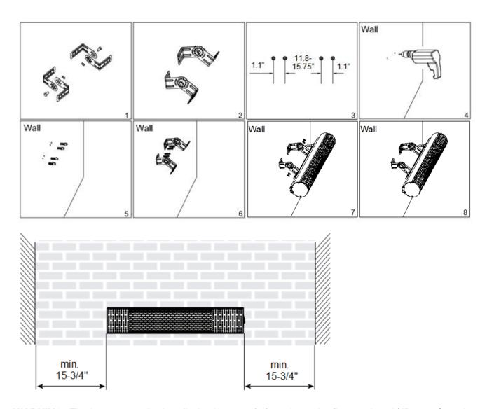
**WARNING:** The heater must be installed at least 6-1/4 feet above the floor and 15-3/4" away from the walls on both sides. The power cable must not pass through the heater while installing.
