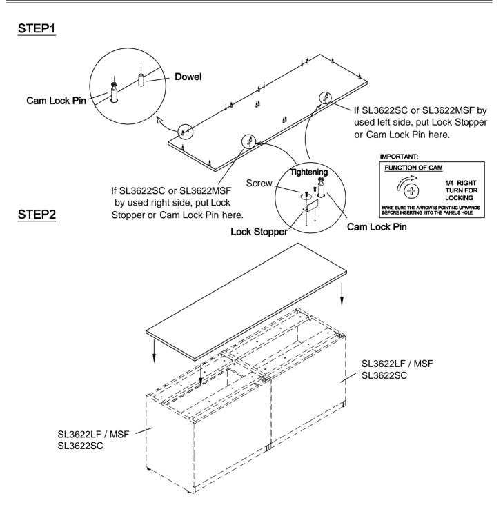
Use Cam Lock Pin and Dowel to attach top as provided with Lateral file or Storage.
