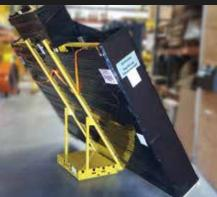
Unlike standard hand trucks, the objects can be moved in any direction, making long objects easier to move.
