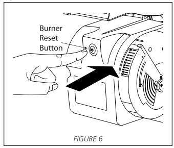
**RESETTING THE SAFETY THERMOSTAT:** Safety thermostat operation is identified by an indicator light. Refer to Figure 2. Identify and remove the cause that triggered the safety thermostat. Press the reset button located at the back of the heater all the way.
