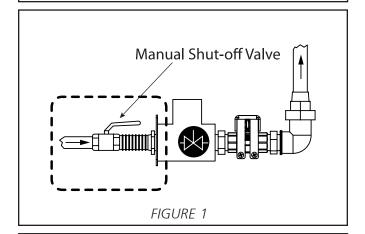
**CAUTION:** If the heater is connected to natural gas, installation must be compliant with local laws and, in case of no specific regulations, refer to the national regulation on gas fuel ANSI Z223.1/NFPA 54 and to the natural gas and propane gas installation regulation CSAB149.1.
