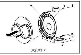
2. Remove the plates, which close the inspection openings, by removing the screws. See Figure 8.
