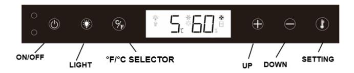
**NOTE:** Pressing the **ON/OFF** key once can switch off the audible alarm when the alarm is on.
