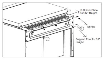
5. Reusing the original screws, install the kick plate and supporting feet for 34.25" height,
