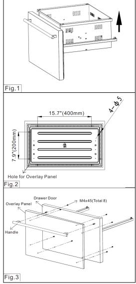
Peel back the gaskets, then align the left and right side channels with the tracks in the cabinet. Ensuring an even track engagement on both sides, gently push the drawer into the cabinet until it stops.
