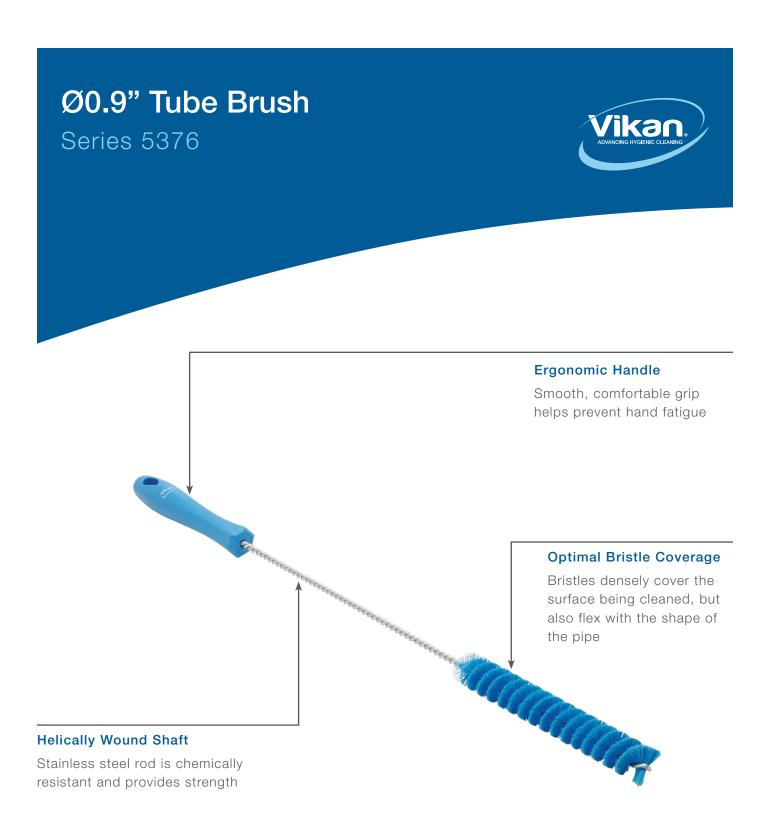
This tube brush with a 0.9 inch diameter is great for cleaning pipes and narrow spaces between machinery. Made from FDA-compliant materials, this piece is fit for inclusion into any color-coding program.
