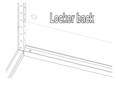
2B-2 With the back inserted install one 8709 screw on each side of the back about half way up. Note holes are to align to make sure back is in proper position.
