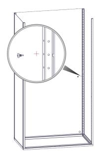
2C-1 Insert cast corner pieces of locker bottom into the side channels.
