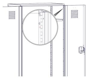
Assembly is now complete. Lockers to be floor and wall anchored and must <u>be plumb and level</u> after anchoring before use.
