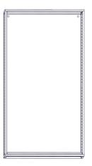
2F-Install screws to locker back at U cut locations (6 inch intervals) on each side.
