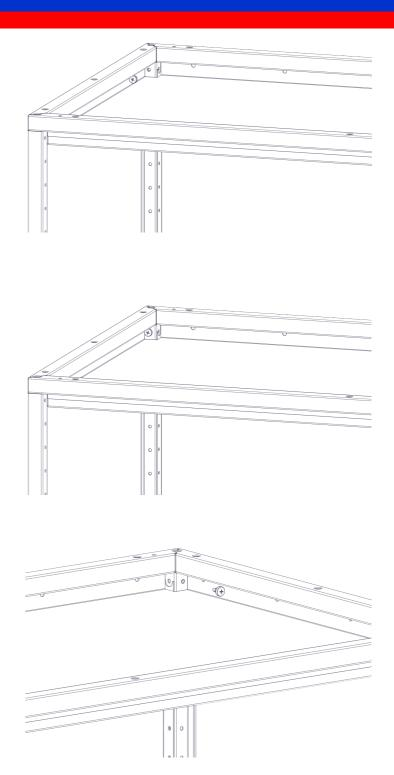
2C-2 Install one screw into each corner of the locker bottom as shown.
