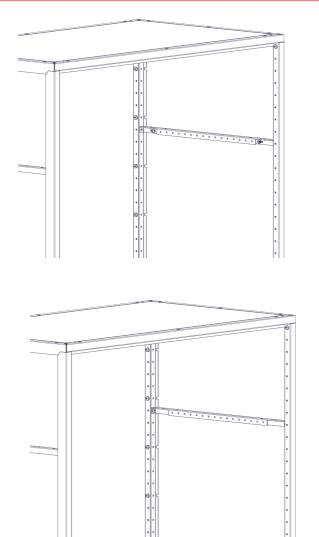
2G-2 Insert shelf and attach shelf to rails using one rivet in each corner.
