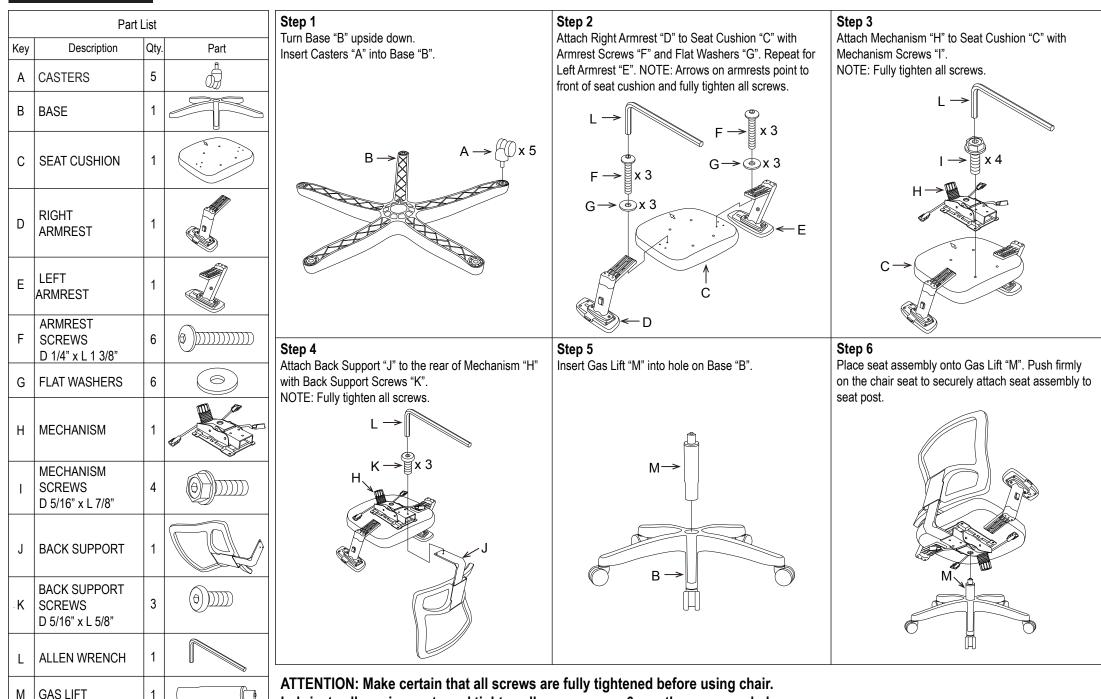
Lubricate all moving parts and tighten all screws every 6 months or as needed.
