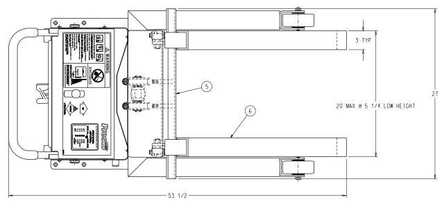
FORKS CAN BE SPREAD WIDER UP TO 26 O.D. @ A LOW HEIGHT OF 6  $1/4^{\prime\prime}$
