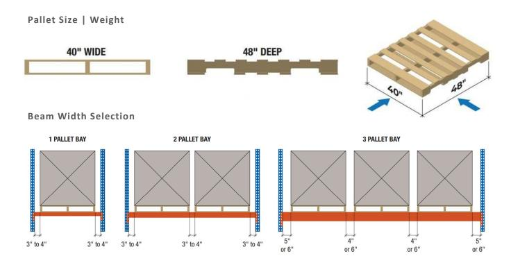
Selecting the correct beam width for your application use is determined by adding the width(s) of your pallet loads.
