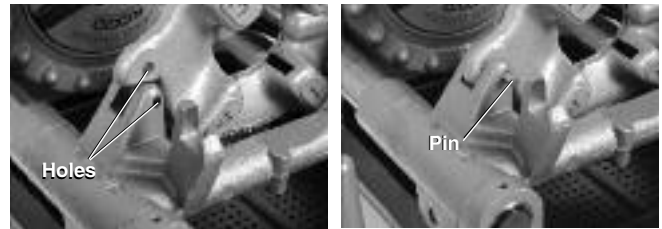
Figure 26 – Retaining LH Die Head in Place
