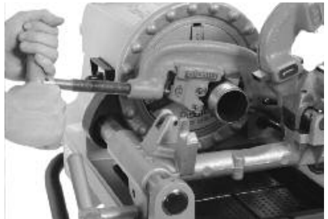
Figure 22 – Cutting Pipe with Cutter
