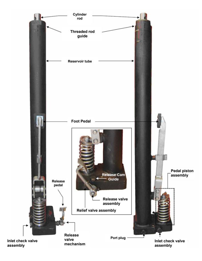
Release Valve and High Pressure Relief Valve Assemblies
