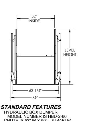
CHUTE IS 52" W X 50" L (USABLE) DUMPER CAPACITY IS 2000 LBS. DUMP HEIGHT IS 60" HOLD DOWN WILL ACCEPT BOXES 18" TO 50" HIGH W/ HOLES EVERY 2" FRAME WIDTH IS 69" FRAME LENGTH IS 68 1/2" LEVEL HEIGHT IS 77" ROTATED HEIGHT IS 149 1/2" DUMP ANGLE IS 45° CHROME PLATED CYLINDER WITH EMERGENCY STOP VELOCITY FUSE PAINT IS VESTIL ROYAL BLUE WARNING: CHECK STATE AND LOCAL CODES!!
