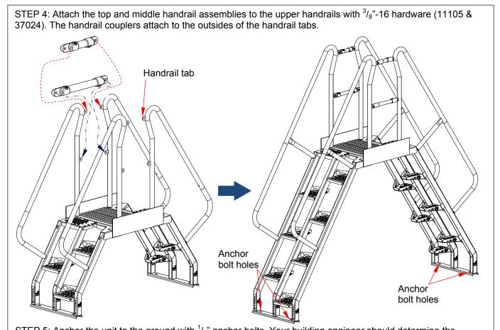
STEP 5: Anchor the unit to the ground with  $^{1}/_{2}$ " anchor bolts. Your building engineer should determine the necessary length of the bolts. Mark the floor with the locations of the anchor bolt holes in the mounting plates. Then install the anchors and solidly fasten the ladder to the ground.
