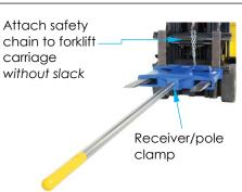
**Step 4**: Raise the forks only as high as necessary to lift the roll of carpet off of the ground and to avoid contact with objects during transport. DO NOT leave a raised roll unattended. Always unload the carpet ram before leaving the forklift.
