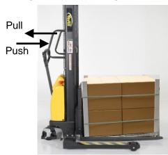
Always avoid sudden stops, quick turns or quick starts to prevent accidental tipping or shifting of the load.
