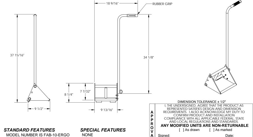
MODEL NUMBER IS FAB-10-ERGO CHOCK WIDTH IS 9 13/16" **OVERALL WIDTH IS 18 9/16"** CHOCK LENGTH IS 9 1/2" OVERALL HEIGHT IS 37 15/16" CHOCK HEIGHT IS 7 7/32" HANDLE COMES WITH RUBBER GRIP SHIPS KNOCKED DOWN 10' CHAIN INCLUDED (NOT SHOWN)
