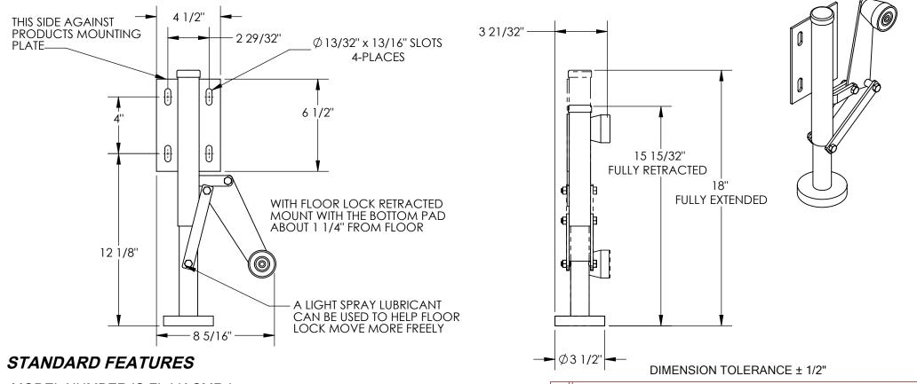
MODEL NUMBER IS FL-LK-SMR-L OVERALL WIDTH IS 8 5/16" OVERALL HEIGHT IS 18" FOOT PAD Ø3 1/2" GROUND TO HOLE 12 1/8"
