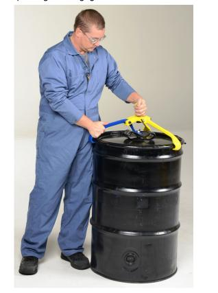
To release the Drum-Grab from the drum, pull the lifting ring towards the rim hook of the pivoting arm to compress the rubber spring. When the spring is sufficiently compressed, separate the rim hook from the rim; then lift the pivoting arm and slowly allow the spring to recoil. The fixed arms can now disengage the rim.
