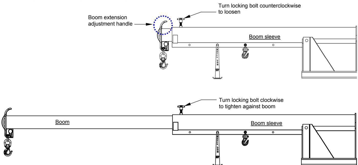
4. **[OBT models only]** Adjust the boom angle, if necessary, to accommodate the load. To safely perform the adjustment process requires *at least* 2 people:
