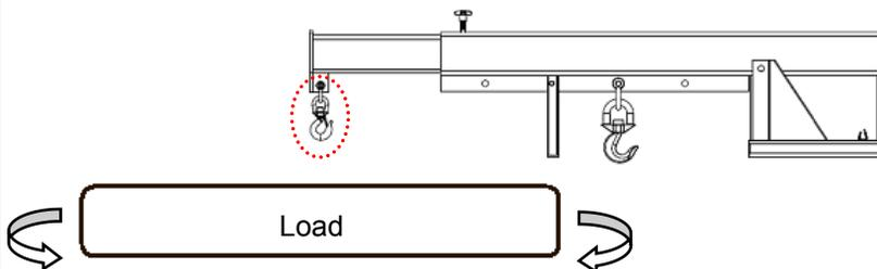
Load attached to both hooks: load rotation minimized
