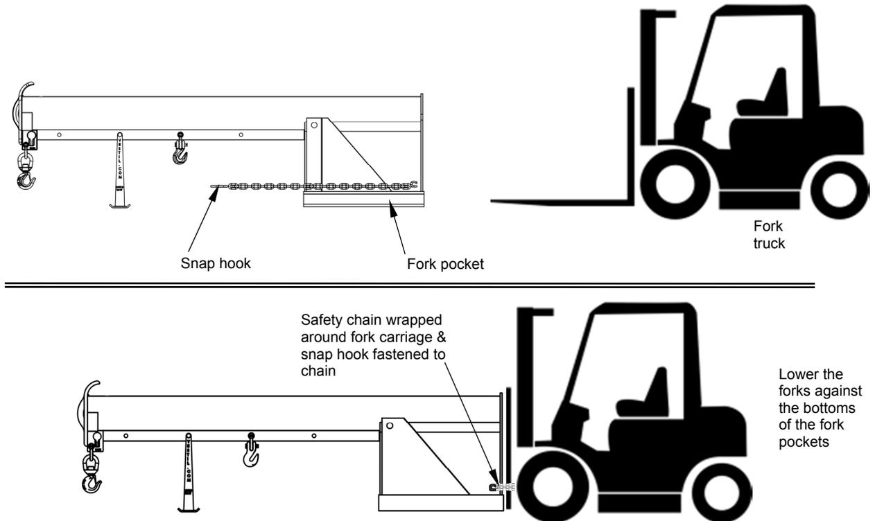
2. Securely connect the boom to the carriage of the forklift with the safety chain.
