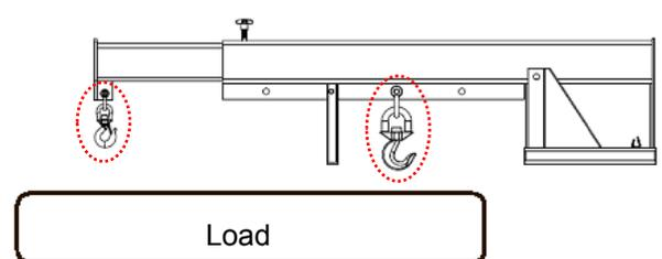
**Test the stability of the load in the rigging.** Raise the forks *slowly* to minimize load movement. Raise the forks until the load is entirely suspended from the boom. Watch the load and boom closely for *either* of the following issues: 1) Load sliding in rigging; or 2) Boom sliding towards tips of forks. If you notice either issue, immediately lower the forks and adjust the rigging. Retest the stability of the load in the rigging
