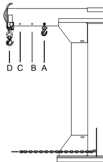
Center of gravity has both a horizontal component and a vertical component. The *vertical* center of gravity (VCG) lies along a line 38 inches (~97 cm) from the bottom edges of the fork pockets. Similarly, the *horizontal* center of gravity (HCG) is located 8 inches (~20cm) from the front edge of the vertical support.
