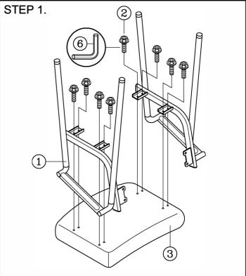
Align back of (3) seat to holes of (1) steel frames . Attach with (2) steel frame screws, but do not tighten completely.
