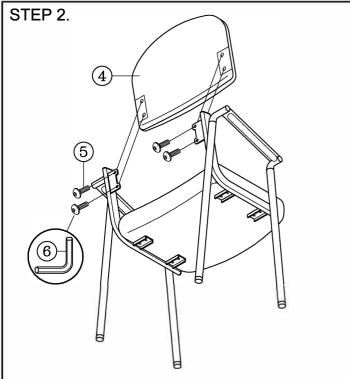
Align (4) backrest to (1) steel frames as shown. Attach with (5) backrest screws . Adjust (1) steel frames until properly aligned. Securely tighten backrest screws and steel frame screws of (3) seat.
