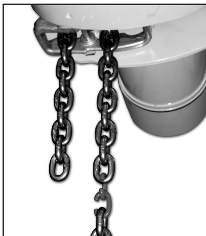
Figure 5-4. Installing Coil Load Chain Using Two "C" Links (1/4, 1/2 & 1 ton hoists)
