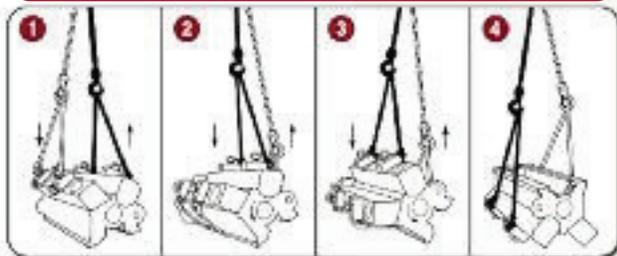
Engine block is raised straight up (1) by special cylinder lift rings, then rotated approximately 45° until one load hook (2) supports total weight. Sling is guided under block and attached to free hook (3). Hoist is then reversed (4) until block is inverted.
