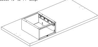
**3.** Secure the housing to the top, using four #14-3/4" hex head slotted wood screws (Ref. No. 11).
