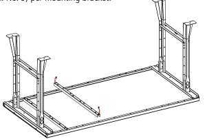
NOTE: One set of mounting brackets comes with the standard steel top workbench. Additional sets of mounting brackets must be purchased separately if attaching more than one drawer or attaching a drawer to a modular workbench. **3.** Attach the drawer housing to the mounting brackets. Secure with four 1/4"-20 x 5/8" bolts.
