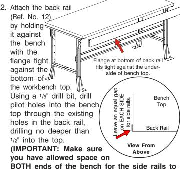
BOTH ends of the bench for the side rails to slip underneath the back rail.) Attach with eight #14 x 3/4" slotted wood screws.
