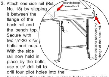
bench top through the existing holes in the side rail. Attach with four #14 x <sup>3</sup>/<sub>4</sub>" slotted wood screws. Repeat this procedure to attach the second side rail.
