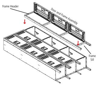
**8.** If joining a three wide unit beside another unit, temporarily install a bolt and nut into the third and sixth holes down from the top of the outer frames that will be joined to the adjacent locker frames. The center locker frame can be bolted complete. If the locker is just a stand alone three wide unit, finish attaching the frames using thirty eight bolts and nuts. Check and tighten all permanent bolts.
