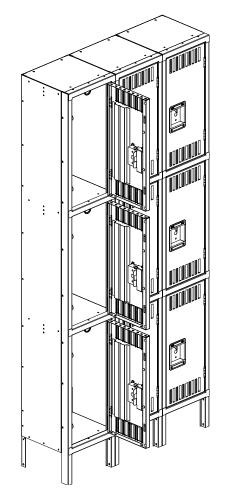
**10.** Anchor units to wall or floor. The units are not intended to stand free and may topple if not secured. Units standing back to back should be bolted back to back.
