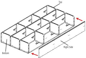
**6.** If the locker has legs, insert the leg into the corner between the bottom and the side as shown.
