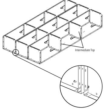
**5.** Bolt the right side (Ref. No. 6) to the back so that side flange fits around the back, then attach the side to the top, bottom, and intermediate top. Use nineteen bolts and nuts (twenty one for a unit without legs) to secure in place.
