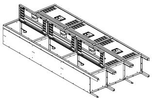
**9.** Stand the unit upright and place in the desired location. Remove temporary bolts in frames and bolt to adjacent units together through frames.
