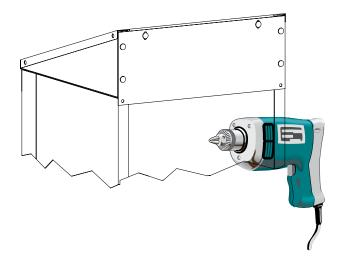
**11.** Install #8-32 x  $^{1}/^{2}$ " bolts and nuts in the holes you just drilled.
