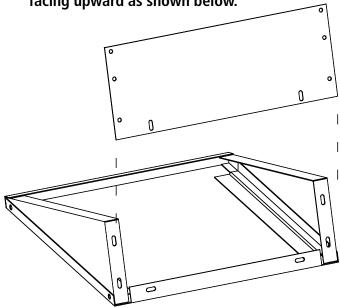
**5.** Fasten the back to the sides with four #8-32 x <sup>1</sup>/2" bolts (Ref. No. 5) and nuts (Ref. No. 6).
