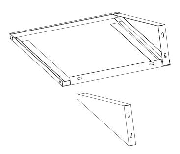
**4.** Place the back plate (Ref. No. 3) against the flanges on the outside of the top and sides.
