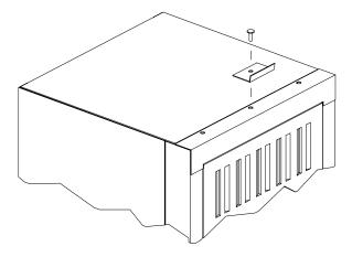
NOTE: On some locker units, the existing hole may contain a rivet. If so, use a drill with a <sup>3</sup>/16" bit to remove the rivet before installing the clips.
