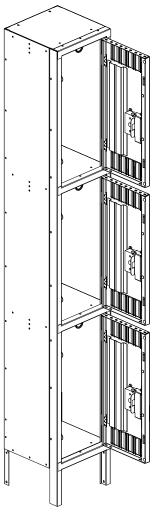
**10.** Anchor units to wall or floor. The units are not intended to stand free and may topple if not secured. Units standing back to back should be bolted back to back.
