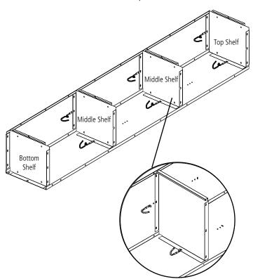
**5.** Bolt the right side (Ref. No. 6) to the back so that the side flange fits around the back also attaching to the top, middle and bottom shelves using twenty-two nuts and bolts if the locker has no legs and twenty-four nuts and bolts for a locker with legs. Attach the remaining hooks to the right side over the flange of the shelves using two nuts and bolts on each hook.
