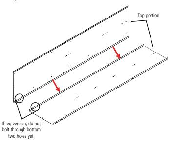
**4.** Bolt the top, middle levels and bottom (Ref. No. 4) to the back and side using four bolts and nuts each. Coat hooks will need to be attached over the flange of the shelves as shown. Use two bolts and nuts per each coat hook.
