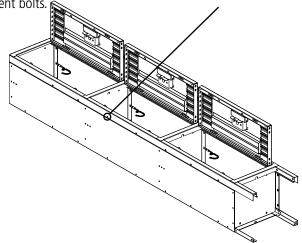
**9.** Stand the unit upright and place in the desired location. Remove temporary bolts in frames and bolt to adjacent units together through frames.
