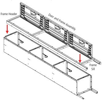
**8.** If joining units side by side, temporarily install only one bolt and nut in the frame(s) that will be joined to the adjacent locker frame(s). If locker is just a single unit, finish attaching the frame using twenty bolts and nuts. Check and tighten all permanent bolts.
