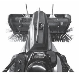
To adjust brush angle: Lift the lever; Turn the brush in the desired direction; Release the lever and ensure the lever is latched in place.
