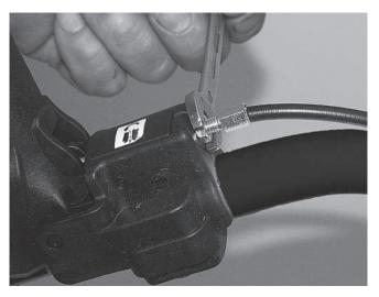
Tighten the nut. Check the adjustment by pressing the lever down.
