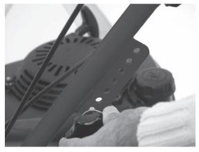
Loosen the knob on both sides and choose the desired position
