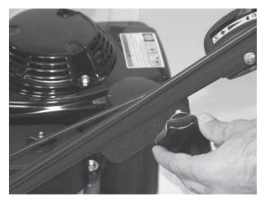
You can fold the handlebar forward to save space when storing.
