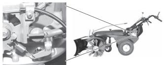
Pull starter coil. Stand behind the handlebars. Do not press any levers.
