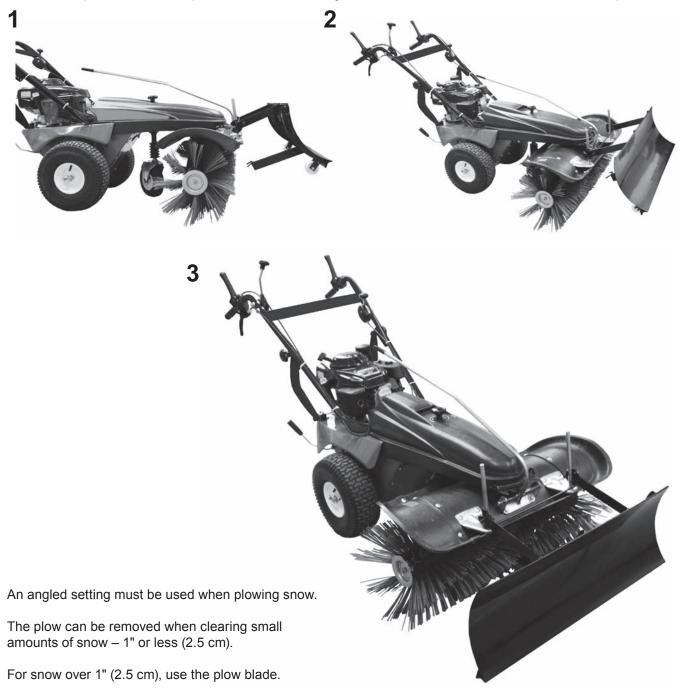
The rotary broom can clear a maximum of 5-1/2" (14 cm) of snow in one pass. If snow is heavy, the capacity will be less.
