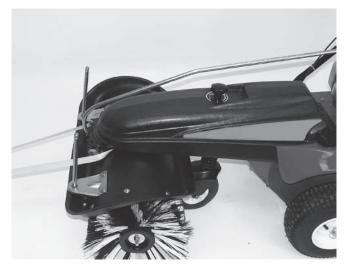
Always use two straps on the rear axle; one on each side.
