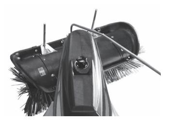
If you use a plow, an angled direction must be used. Shown below: Ejection to the left.
