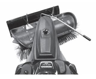
A sideways setting is recommended if using the optional debris collector. This will allow sweeping against a wall or curb. (Debris collector box is an optional accessory).
