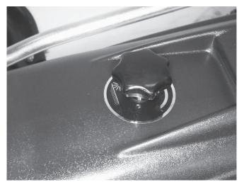
Lower the brush by turning the knob in the direction of the "minus" arrow until it just touches the floor. Turn the knob three more turns and the brush height is just right for sweeping.
