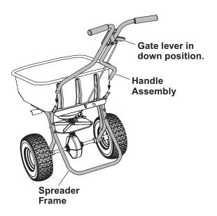
5. Secure with the 1/4" x 1-3/8" cap screws and 1/4" locknuts from the hardware kit.
