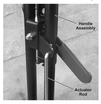
4. With the gate lever in the down position, slide the handle assembly onto the spreader frame.
