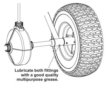
NOTE: Gears and axles must be lubricated and greased every 20 hours of use.
