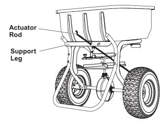
3. Attach the actuator rod to the handle assembly.
