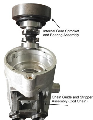
Image 18 Removing internal gear, chain sprocket and ball bearing.
