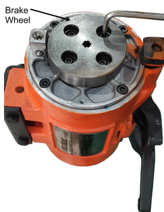
Image 15 Removing Cap Screw Securing Bearing Clamp Plate
