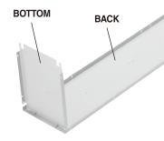
2. Bolt on side with bend in rear and facing in. Omit 2 bolts near bottom rear for legs. Install shelf by bolting to side with bend facing down and 45° bend in front. (See Section 8 Punching Patterns for single, double and 6-tier shelf hole locations.)
