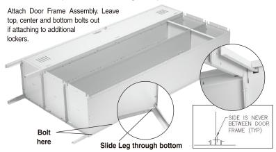
7. Bolt locker foot to leg. Stand locker in place. Level them and adjust rear legs to touch floor and tighten bolts. Floor anchor not included. Bolt banks of lockers together using holes omitted in step #5.
