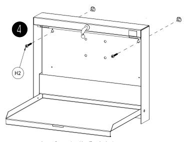
Insert Screws into Kap Toggle Anchor . Do not tighten all the way. Mount Wall Hung Desk over these two screws and tighten.
