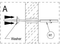
Push Kap Toggle thru drilled hole
