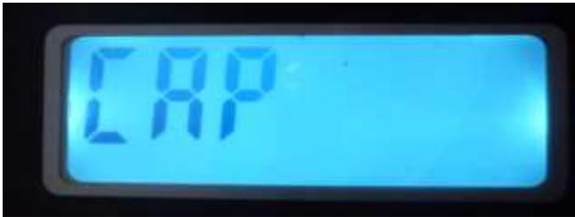
**Step 6.** press "UNIT" to change capacity data 5000 ( press "ZERO" to make 5→5000 ) (as below) ,then press "HOLD" for confirming. ( coz this NP771-3TH's capacity is 5000lbs)
