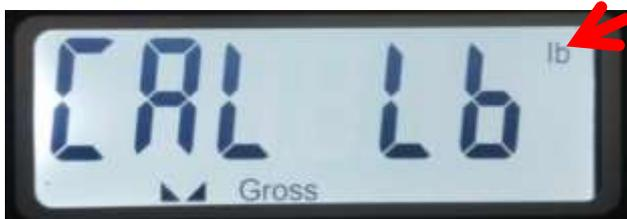
**Notes:** if the code shown as below , that means the weight unit is “kg” but not “lb” . if you want “lb” as weight unit in system, please press “UNIT” to change kg into “lb” (go back hown as the above picture).
