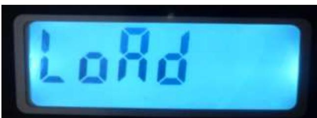
**Step 8.** Press "UNIT" to make weight data around "1100"(as below). Then press "HOLD" for confirming,
