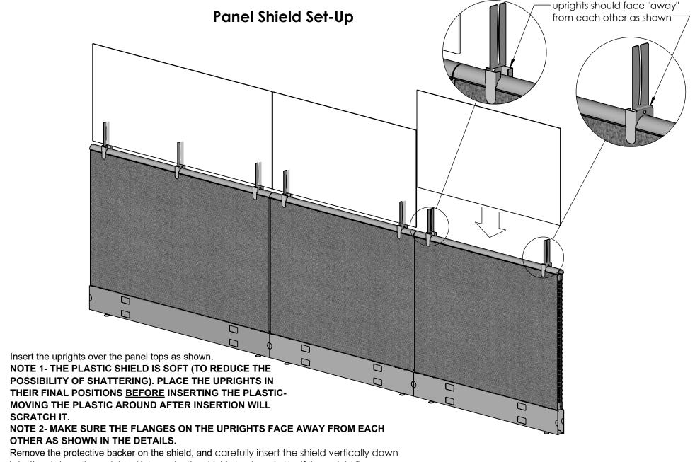
Remove the protective backer on the shield, and carefully insert the shield vertically dowr into the slots on the uprights. Note again- the shield stands up better if the upright flanges face away from each other.
