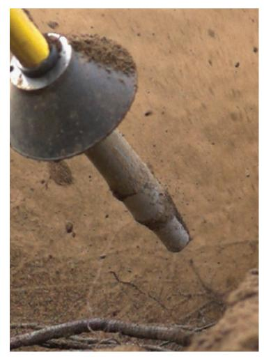
Supersonic Nozzle: Soil fractures from stress (force per unit area) applied to its surface. Focusing this force on a small unit area results in faster, and more efficient soil excavation. As shown in the diagrams above, air exiting from an open pipe, or from a conventional nozzle, expands rapidly outward, across 3 to 4 times the unit area, versus
