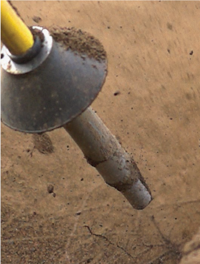
Unfocused air flow from improperly designed nozzle.
