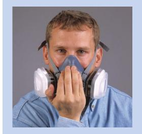
Cover the opening in the exhalation valve cover with your hand. Be careful not to disturb the position of the respirator. Exhale gently. If the facepiece bulges slightly and no air leaks are detected between your face and the facepiece, proper seal has been obtained.\*
