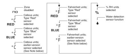
**Note:** Sensor types ("Red", "Blue" or plain "F or "C) refer to the Zone programming required for the type of sensor used:
