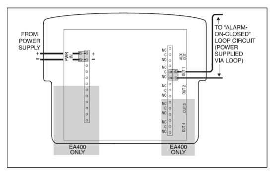
Figure 8. Typical Alarm Loop Wiring Configuration (External Power)
