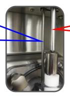
Arm moves up and down and tells machine when product is being dispensed.
