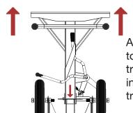
Allow the stand to rise to the height of the trailer. Replace the pin in the nearest hole. The trailer is now stabilized.
