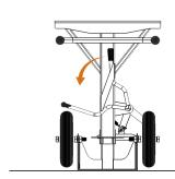
Place light weight on foot stand. Rotate the handle counter clockwise to disengage the pin and allow the stand height to change.
