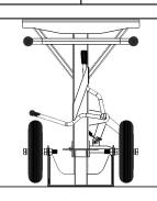
To remove the stand, remove the pin and press down on the foot stand to lower the stand. Once stand is lowered, replace pin. Pull and roll the stand out of the way before moving the trailer.
