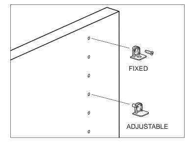
Slide the shelf into place over the Metal Flanges and push down until fully seated.
