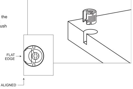
For a Fixed Shelf or Top, install the metal flange using a System (Varianta) Screw as shown. DO NOT over tighten!
