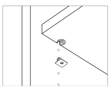
Install four Plastic Housings (H1) into each shelf. Attach a Book Stop (H2) to each Fixed/Adjustable Shelf (E) using five Panhead Screws (H3) in the pre-drilled holes.
