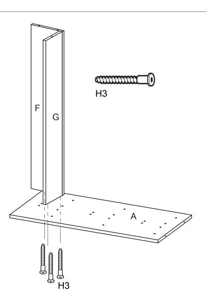
Once all six shelf assemblies are attached, align Right Side (B) onto main assembly. Secure in place using eighteen #8x50 Confirmat Screws (H3)- two for each Shelf Back (F) and one for each Shelf Bottom (G).
