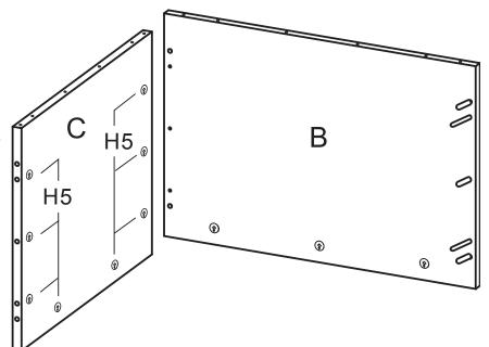
Insert eight Minifix Cams (H5) into a Side Panel (C) facing out. Position the Side Panel onto the bolts and dowels of the Back Panel (B) and turn cams clockwise to lock in place.
