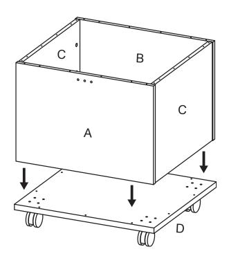
From the hardware included with the Book Drop Bag\*, take four Corner Clips and attach to each corner of unit using 1" Panhead Screws (H7) in the predrilled holes.
