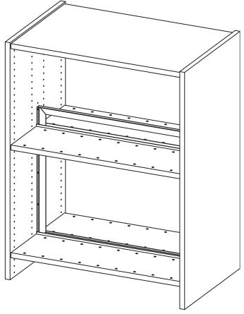
Insert the Divider Wires (H8) into the pre-drilled holes of the upper surface of the Shelves (D) shown.
