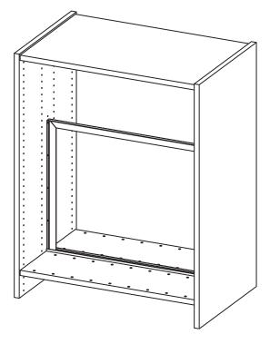
**48" Unit:** Placement of the Shelves (D) is optional. Allow room between shelves to accommodate the Wire Dividers. Push 16 Tab-V Shelf Pins (H7) into the Left Side Panel (A) and the Right Side Panel (B) at the preferred height.
