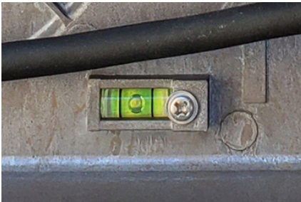
Incorporated level system in fixture
