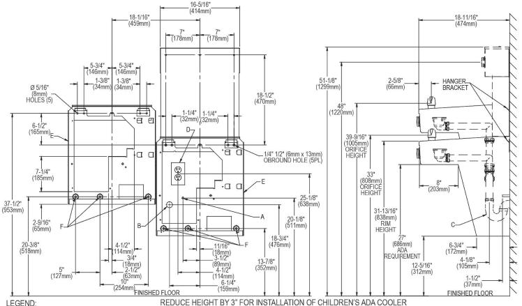
A = Recommended Water Supply location. Shut-off Valve (not furnished) to accept 3/8" O.D. unplated copper tube. Up to 3" (76mm) maximum out from wall. B = Recommended Waste Outlet location. To accommodate 1-1/2" nominal drain. Drain stub 2" (51mm) out from wall.
